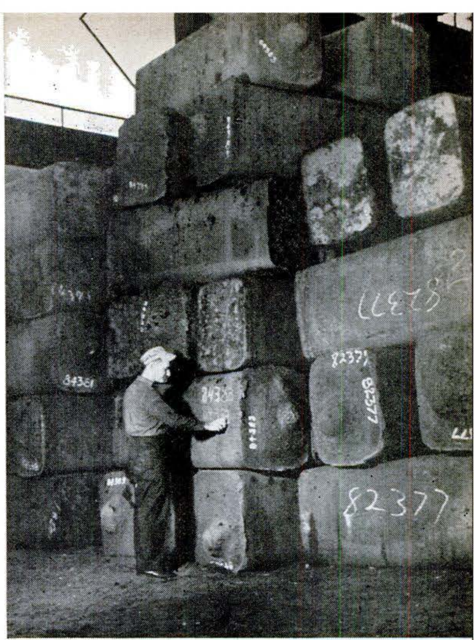
Here are steel ingots waiting to be made into rod, wire, and nails. Each 25- by 30-inch ingot is seven feet long, weighs six or seven tons.
